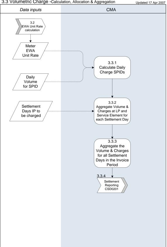
3.3 Volumetric Charge -Calculation, Allocation & Aggregation
